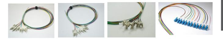
Fibre Optic pigtails are essential when terminating cables within a splice enclosure by either using a fusion splicer or mechanical splicing. Using pre-polished assemblies can reduce the risk of poor connector termination and therefor loss. Cables terminated within a production facility will give a higher performance than cables terminated on site.
